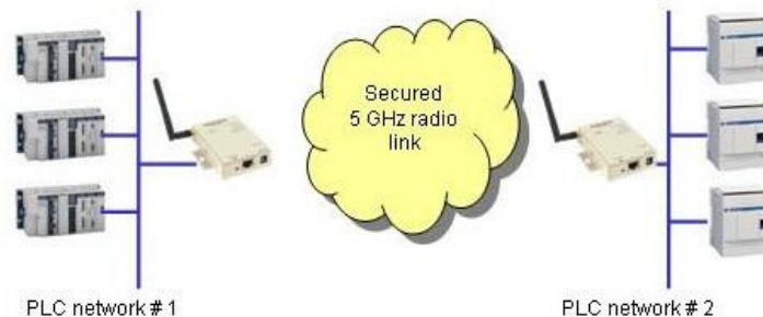
INTERCONNECTION BETWEEN TWO ETHERNET NETWORKS
