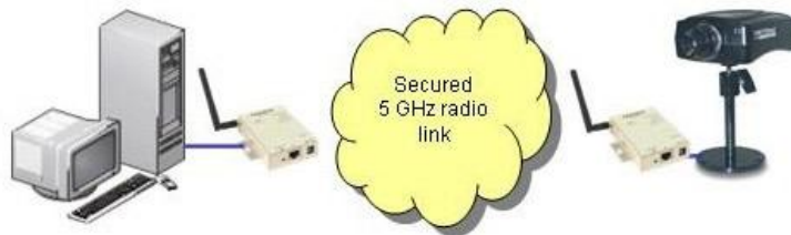
RJ45 ETHERNET CABLE REPLACEMENT BETWEEN TWO EQUIPMENTS
