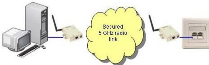
OFFICE NETWORK CABLE REPLACEMENT
