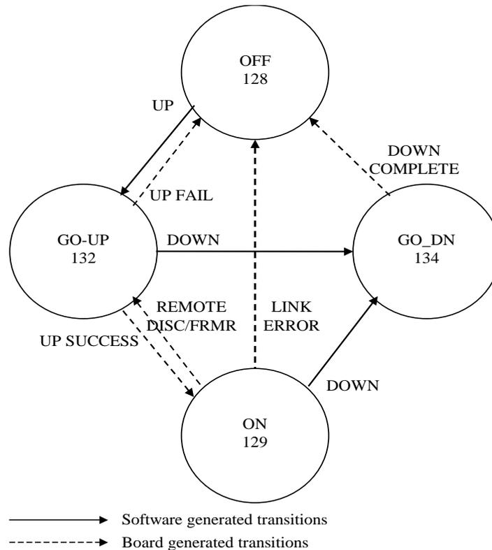
There are four states in the driver: `MCX_LINK_OFF`, `MCX_LINK_ON`, `MCX_LINK_GO_UP`, `MCX_LINK_GO_DN`. The state changes can result from a user program action (calling `PRCTL`) or from a card or remote action (link error detection, close by remote).
