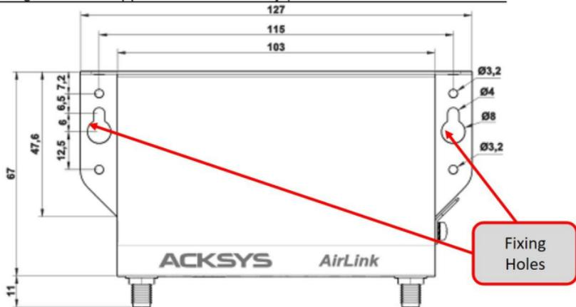
Moreover, it is possible to mount the product on a DIN RAIL using the **WL-FIX-RD2** kit
