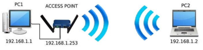
Set up the PC2 Wireless network interface according to the default parameters of the ACKSYS AP device (802.11gn, SSID "acksys", no security).
