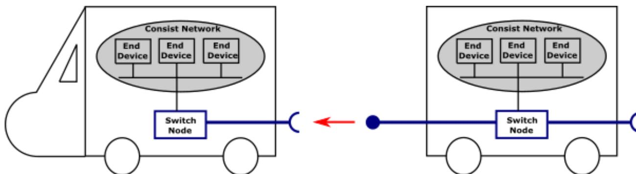
Since network wiring between carriages may be difficult or often impossible, particularly in case of refurbishment operations because of aging or poor-quality connectors, WiFi has naturally established itself as the most efficient solution by allowing redundancy, reliability and high-speed networking.
