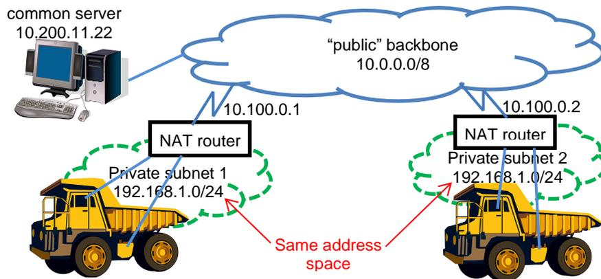
In the case of a NAT/PAT router, the network is split in two “zones”: the **public zone** which is materialized by the backbone, and where a central administration gives out “public” IP addresses; and the **private zone** where the administrator can assign IP addresses without the knowledge of IP addresses outside.
