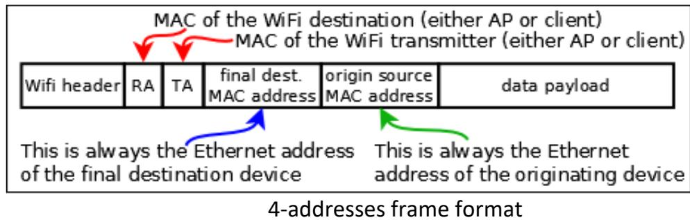
In this solution to the bridging problem, the client bridge and the AP encapsulate both data and Ethernet MAC addresses in the Wi-fi frame, adding both the AP and the client Wi-Fi MAC addresses. So, the frame can reach its Wi-Fi destination, which removes the Wi-Fi addresses and retrieves the original frame unchanged. The same process takes place both ways.
