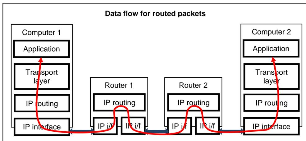
On **WaveOS**, routing is implied when several network interfaces are configured. It can be tuned further in the **ROUTING/FIREWALL** submenu. Please see: [Routing / Firewall](#) chapter.
