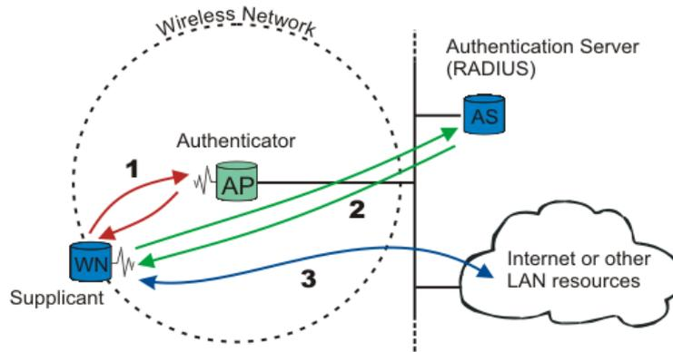
When a wireless node (WN) requests access to a LAN resource, the first step is the physical association between the client and the access point, defining a so-called “access port” (number 1 on the diagram).
