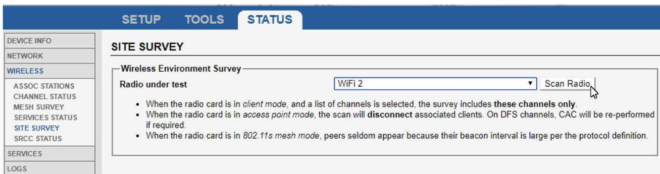
Please note that during the scan period, the radio card can no longer perform the function for which it is programmed. If, for example, it is configured as an Access Point, all associated clients will be temporarily disconnected. Also note that the site survey can work even when the radio card is not activated.
