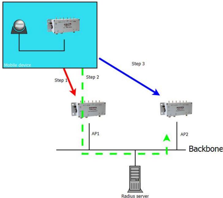
Step 1: The Wi-Fi client associates with AP1 for the first time. In this step the client does a full authentication. The radius server sends the PMK to both AP1 and the Wi-Fi client. AP1 and the Wi-Fi client store the PMK in their local cache.
