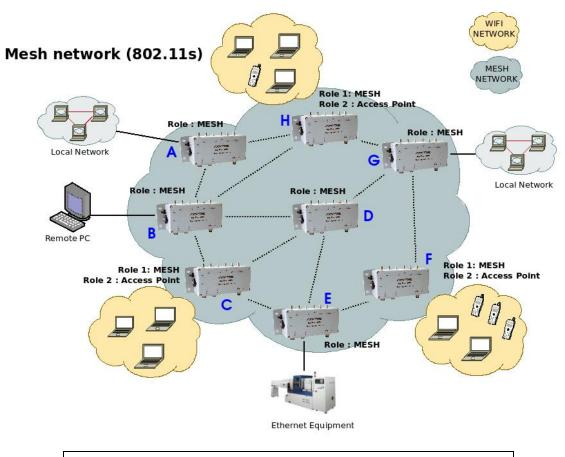
Products A to H can communicate with each other. Products A, B, D, E, G provide Mesh portal functionality. Products C, F, H provide Mesh AP functionality.
