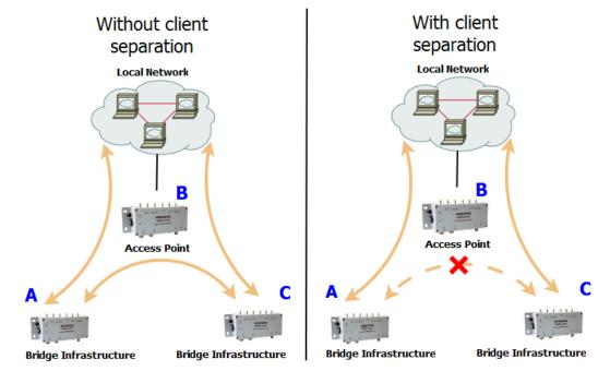
In the infrastructure mode concept, a client is supposed to be a single unit. However the wireless client can bridge several Ethernet devices to a BSS towards the AP, and it still appears as only one device, by converting MAC addresses on the fly (see section V.2.6 Wired to wireless bridging in infrastructure mode).
