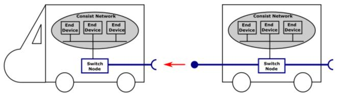
Since network wiring between carriages may be difficult or often impossible, particularly in case of refurbishment operations because of aging or poor-quality connectors, WiFi has naturally established itself as the most efficient solution by allowing redundancy, reliability and high-speed networking.
