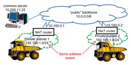
In the case of a NAT/PAT router, the network is split in two "**zones**": the **public zone** which is materialized by the backbone, and where a central administration gives out "public" IP addresses; and the **private zone** where the administrator can assign IP addresses without the knowledge of IP addresses outside.
