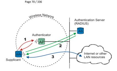
When a wireless node (WN) requests access to a LAN resource, the first step is the physical association between the client and the access point, defining a so-called "access port" (number 1 on the diagram).
