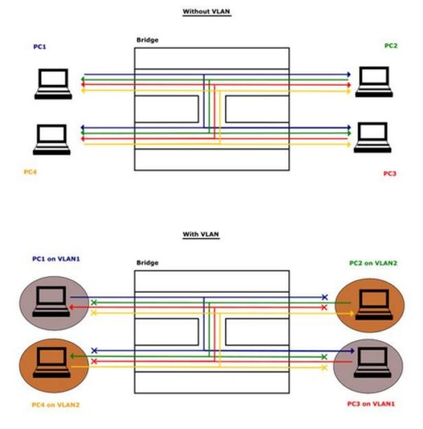
Picture V-3: Computers receive only from computers on the same VLAN
