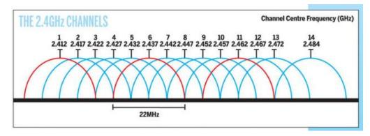
Although the use of "non-overlapping" channels 1, 6, and 11 has limits when products are too close, the 1-6-11 guideline has merit. If transmitter channels are chosen closer than channels 1, 6 and 11 (for example, 1, 4, 7 and 10), overlap between the channels may cause unacceptable degradation of signal quality and throughput.
