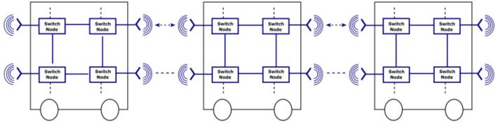
Picture V-9: Example of redundant Ethernet backbone configured with SRCC
