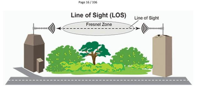
Non-line-of-sight (NLOS) and near-line-of-sight are radio transmissions across a path that is partially obstructed, usually by a physical object in the innermost Fresnel zone.
