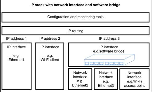
Picture V-8: Example of combined routing/bridging setup
