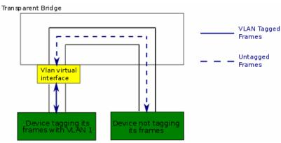
Picture V-7: VLAN tag conversion using a virtual interface
