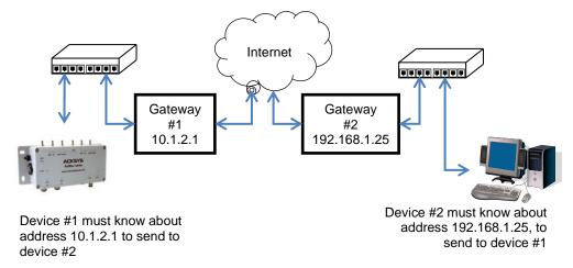
When several routers are available on a single LAN to access various remote LANs, the network devices on the LAN should know about each router's own address and the remote network addresses they lead to. Usually, one of the routers is designated as "default", the other ones are treated as exceptions to this default route.
