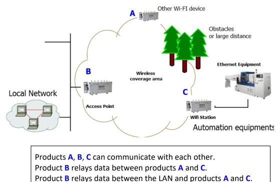
The infrastructure mode provides central connection points for WLAN clients and the AP may also bridge them to a wired network. Prior to any communication, the client must join the WLAN (wireless LAN) by selecting one access point, authenticating and possibly establishing encryption keys.
