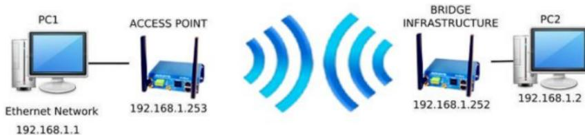
Set up the IP addresses according to the picture above and set the device connected to PC2 to Client (infrastructure) role.
