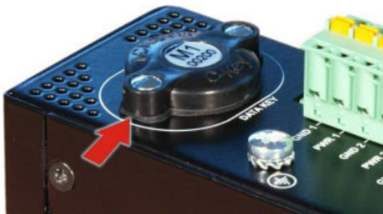
To remove the C-KEY, unscrew the two lateral screws, and then pull the device upward, vertically. If needed, use the screwdriver as a lever, with the help of the notches intended for this purpose at the base of the screw guides.
