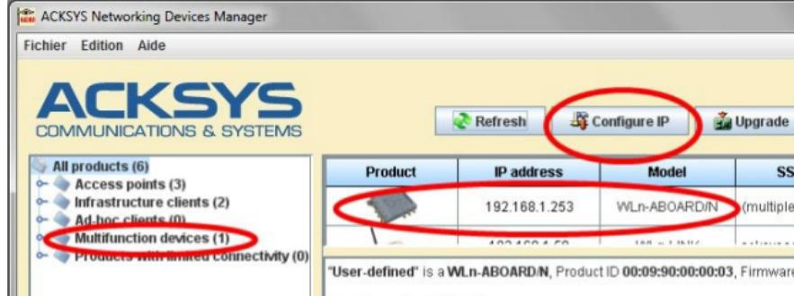
Go directly to step 5 if the default IP address is compatible with your network. Else, select the device and click on the « **Configure IP** » button. You can configure the IP address or activate the DHCP client.
