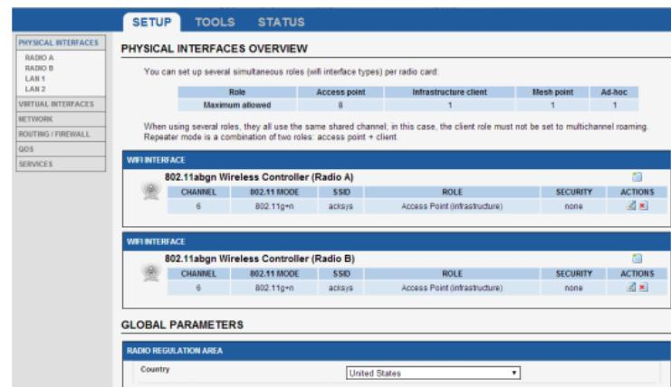
You can select any radio interface to set up its Wi-Fi parameters (alternatively you can navigate to change network and services configuration). Set the following essential parameters:
