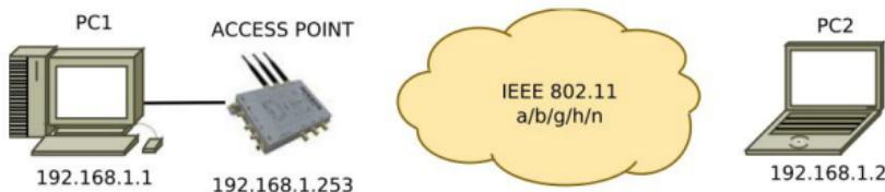
Set up PC2 Wireless network interface according to the default parameters of the ACKSYS AP device (802.11gn, SSID "acksys", no security).
