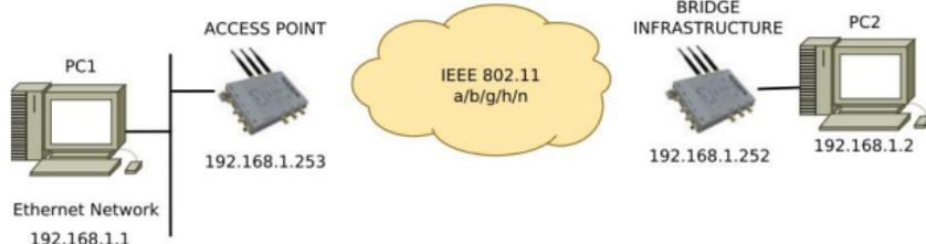
Set up the IP addresses according to the picture above and set the device connected to PC2 to Client (infrastructure) role.
