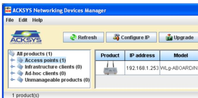
**CAUTION :** the field « Model » is filled with the generic name « WLg-ABOARD/N\_V3 » for products WLg-ABOARD/NI, WLg-ABOARD/NPI, WLg-ABOARD/N\_V3 et WLg-ABOARD/NP\_V3.
