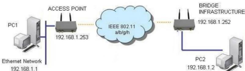
Setup the ACKSYS device connected to PC2 in bridge mode.
