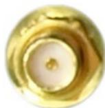
If you don't plug the auxiliary antenna, consider plugging a RP-SMA type antenna terminator.
