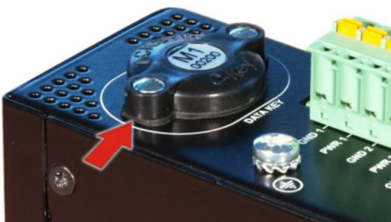
When installing a new C-KEY, be sure that the flattening looks to the rear of the product, then carefully insert the device in the opening, vertically.
