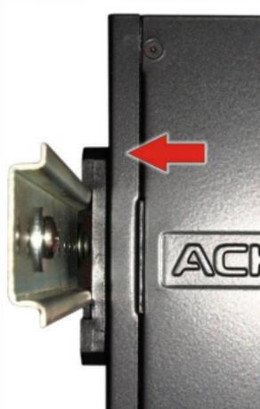
To remove the product from the rail, proceed inversely in the same way: push the device upward, and then, with a rotating movement, pull the upper side of the clip out of the rail, then release the lower side of the clip.
